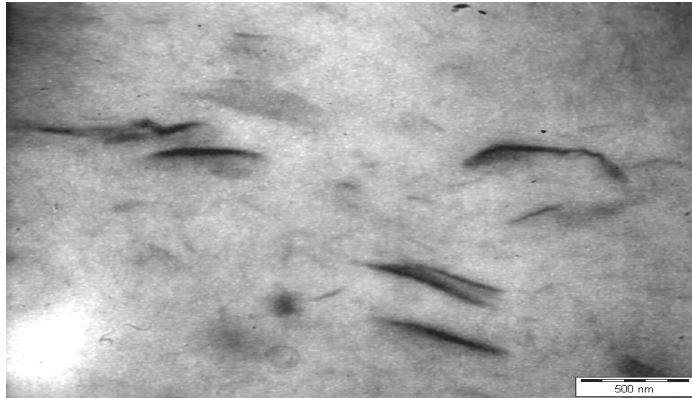
Figure 16: TEM micrograph for 8 phr organoclay-filled ENR nanocomposites.
