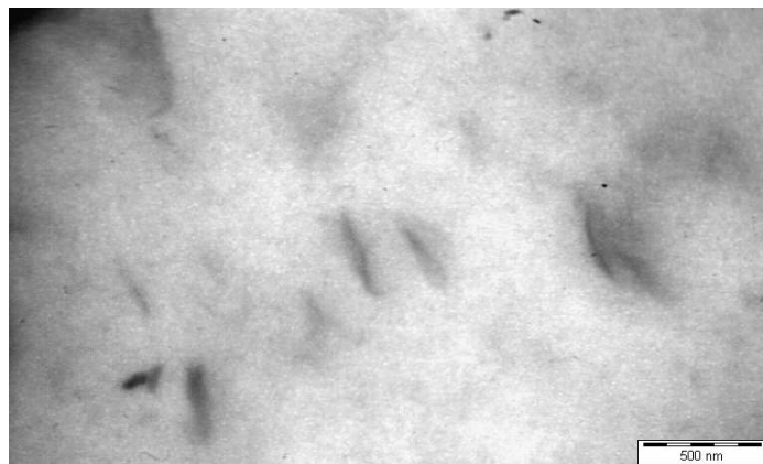
Figure 18: TEM micrograph of NR/organoclay nanocomposites at 2 phr filler loading.
