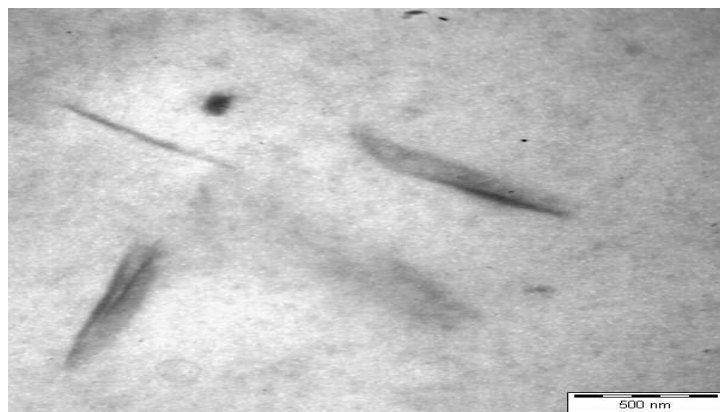
Figure 19: TEM micrograph of NR/organoclay nanocomposites at 8 phr filler loading.
