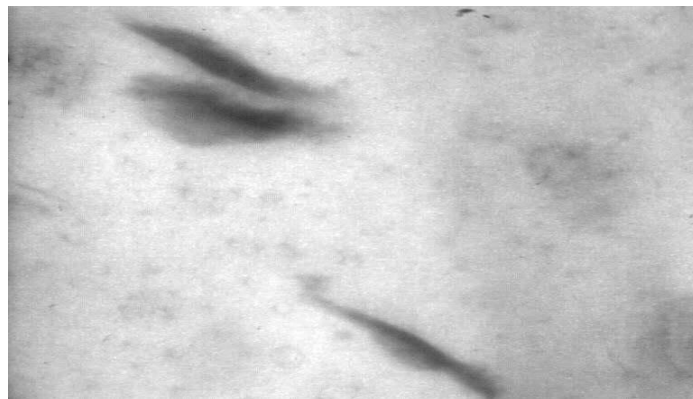
Figure 17: TEM micrograph for 10 phr organoclay-filled ENR nanocomposites.
