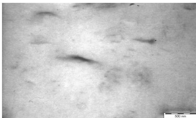
Figure 15: TEM micrograph for 2 phr organoclay-filled ENR nanocomposites.
